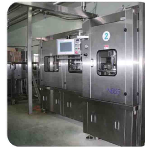
(Filling And Sealing)
